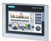
SIMATIC HMI TP700 Comfort, Comfort Panel, touch operation, 7" widescreen TFT display, 16 million colors, PROFINET interface, MPI/PROFIBUS DP interface, 12 MB configuration memory, Windows CE 6.0, configurable from WinCC Comfort V11
